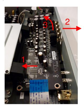
Insert the Vanity<sup>103</sup> module just in reverse order of the analog board removal. Fit the L-shaped holder and fix it with the one screw to the bottom chassis and the one screw to the back panel. This may require some practice.
