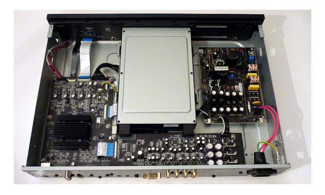
Carefully disconnect the data flat foil cable from the analog board. Release the connector lock first and pull the cable out. Then disconnect also the power cable from the analog board. When both cables are disconnected, remove 3 screws holding the analog board.
