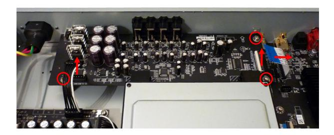
In this step remove the last screw on the metal L-shaped holder and carefully release it from its place. It is necessary to unhook the holder and move the upper end away from the analog board.
