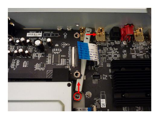
Now the analog board can be removed. Shift the board slightly towards the front side of the player in order to release the RCA connector block from the back panel (1). Then tilt the board with the RCA block upwards while you gently pull the back panel away from the RCA connector (2+3). Then lift the board out of the player.
