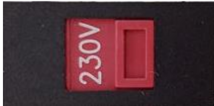
Voltage selector set to 230V
