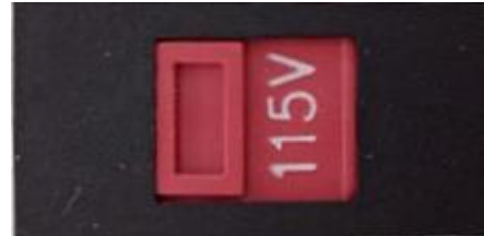
Voltage selector set to 115V
